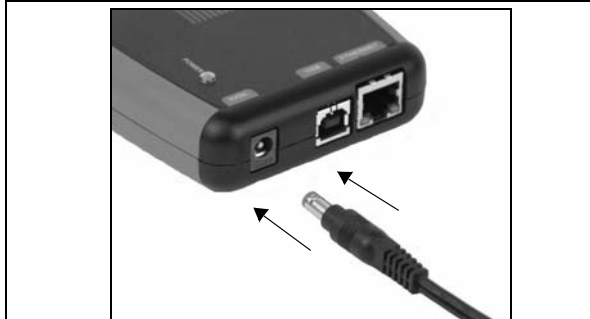
Figure 2-5, Applying Power to XDS560v2 STM
