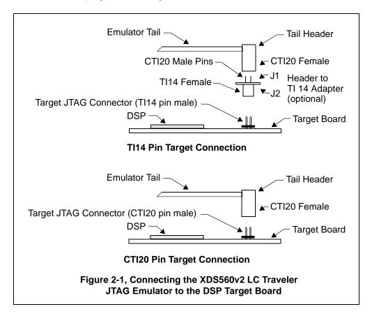
The figure below shows the factory installed configuration with the optional (CTI20 to TI14) adapter installed.
