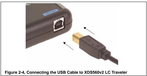
The "PWR" LED (see figure 2-8) on the XDS560v2 LC Traveler should illuminate. After about 45 seconds LED "State 3" should come on. At this point the XDS560v2 LC Traveler has booted its operating system and is ready for connecting via USB.
