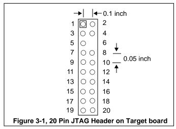
The signals on these pins are shown in the table below.
