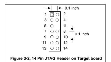
The signals on these pins are shown in the table below.
